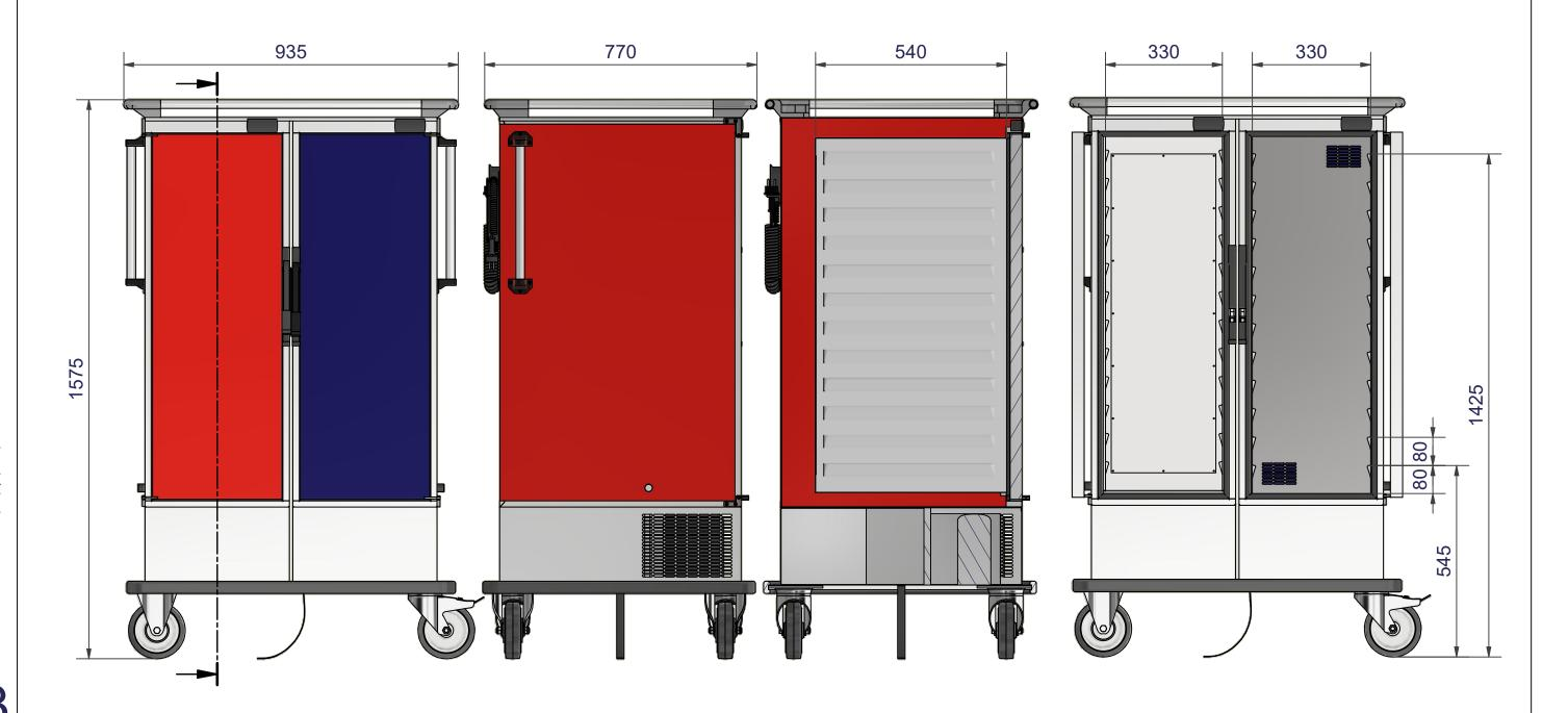
Total weight = 115kg Min working height = 545mm Max working height = 1425mm
