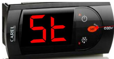
Press and hold Enter until the display shows the set point, then release the button immediately.
